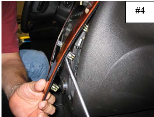
Using a flat head screwdriver concentrate pressure on or around the trim bezels “J” clips
